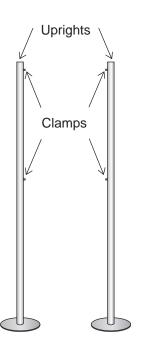
Clamps align onto cut outs of Light Panel
